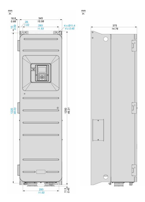
IP55 / UL Type 1 Drive Without Disconnect Switch - Front and Side view
