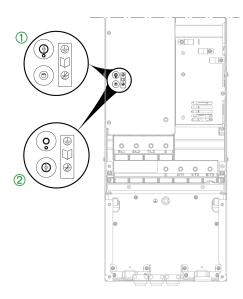
Setting For Frame Size 5S, Frame Size 5Y and Frame Size 6 Products
