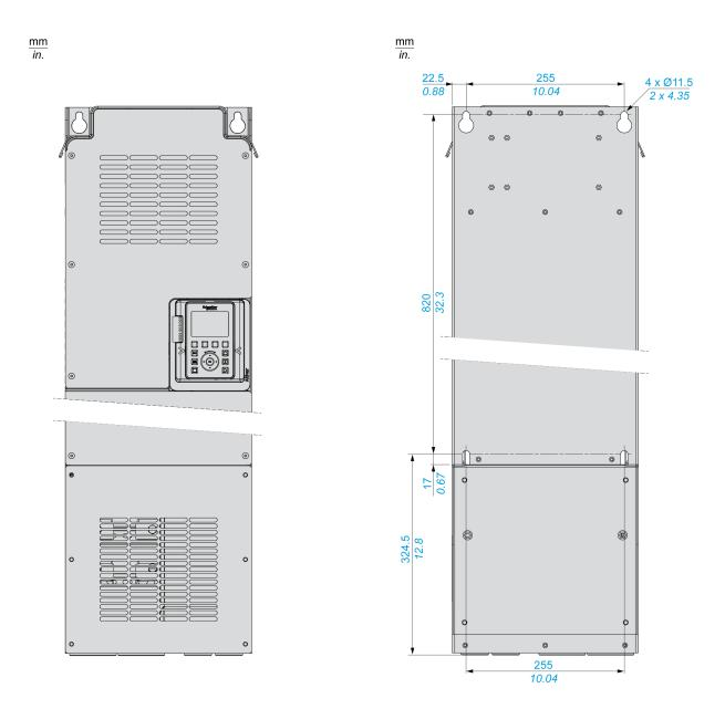
**NOTE:** Lower Conduit Box part VW3A9704 sold separately. This part enables wall mounting of the product. It provides IP21 protection degree on the lower part and UL type 1 protection degree.
