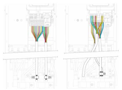
Example: cable path for frame size 3Y for 500-690 V mains voltage
