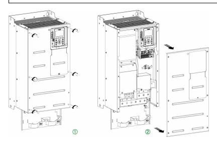
Apply the following instructions to access the terminals on **frame sizes 3Y and 5Y** drives
