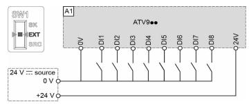
Switch set to **EXT** (Sink External) position **with functional isolation** on digital inputs. This configuration requires the use of 2 external supply units.
