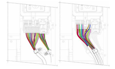
Example: cable path for frame size 5Y for 500-690 V mains voltage
