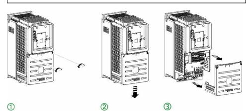
Apply the following instructions to access the terminals on  $\ensuremath{\textit{frame sizes 1 to 3}}\xspace$  IP20 drives
