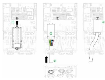
**NOTE:** Cabling plate shown is for frame size 2. Other cabling plates look slightly differs from this one.
