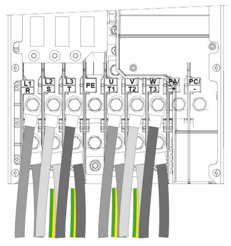
For 4 cable connection, wire the power cables as shown below.
