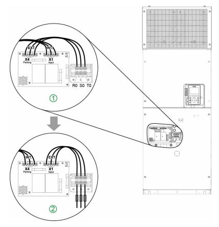
1 Factory wiring: Fans powered internally by R/L1, S/L2, T/L3.
